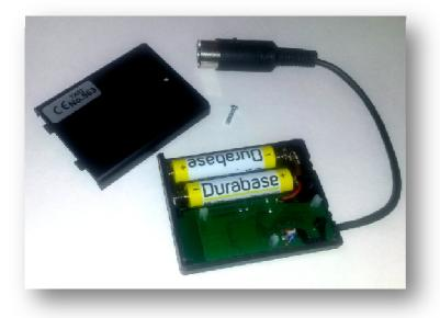
The transmitter runs on two regular AAA batteries. With a small Philips screwdriver, unlock the small screw of the the battery compartment, remove the cover and replace the batteries as shown in the picture. Please observe the correct polarity as shown. Close the cover and put the screw back in place.
