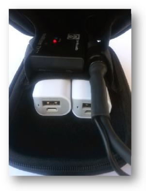
Finally, close the box by pulling up the zippers from the left and right sides. Close the body pack by carefully pushing both USB cables inside the rim of the box. Only the Midi cable leads to the outside from the top center of the belt pack.
