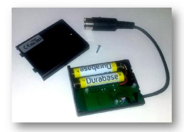
The transmitter has two regular AAA batteries inside. With a small Philips screwdriver, unlock the small screw of the battery compartment, remove the cover and replace the batteries as shown in the picture. Please observe the correct polarity as shown. Close the cover and put the screw back in place (optional).
