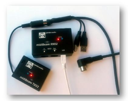
The wireless MIDI receiver RX-02 and the wireless MIDI transmitter TX-02 are shown in the picture below. Connect the MIDI receiver RX-02 with the (supplied) USB mini cable to your computer.
