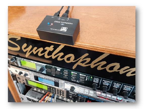
If a connection needs to be made to a hardware synth or a MIDI keyboard, the RX-02 receiver will need power from the USB charger. Connect the charger and the RX-02 using the USB mini cable (included). Finally, use a standard MIDI cable to connect the RX-02 MIDI output to the MIDI input of the keyboard synthesizer or rack mounted hardware synthesizer.
