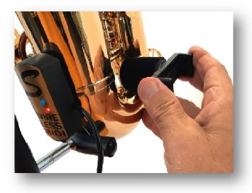
The bracket for the USB power bank is mounted at the low end of the Synthophone. The cylindrical padded mounting device allows for a solid and easy insertion.
