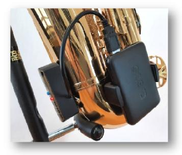
A USB power bank is used to power the Synthophone and the MIDI transmitter "Compact". A fully recharged battery provides up to five hours of wireless operation.
