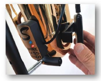
The USB power bank can be removed easily from its bracket and can be recharged using the supplied USB charger. The charging time takes about 4 to 5 hours. While one USB power bank is used on the instrument, the other USB power bank can be recharged.
