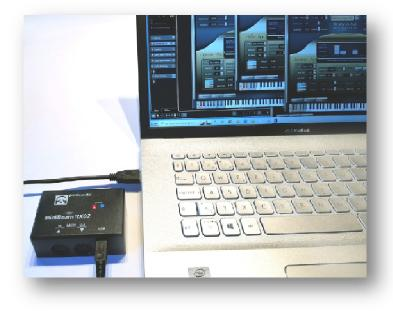
The receiver RX-02 connects to the computer via USB and works without a software driver. It is a "plug and play" device for Windows and MAC operating systems.
